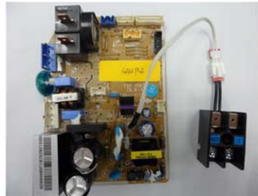
Connection of terminal block and Main PBA
