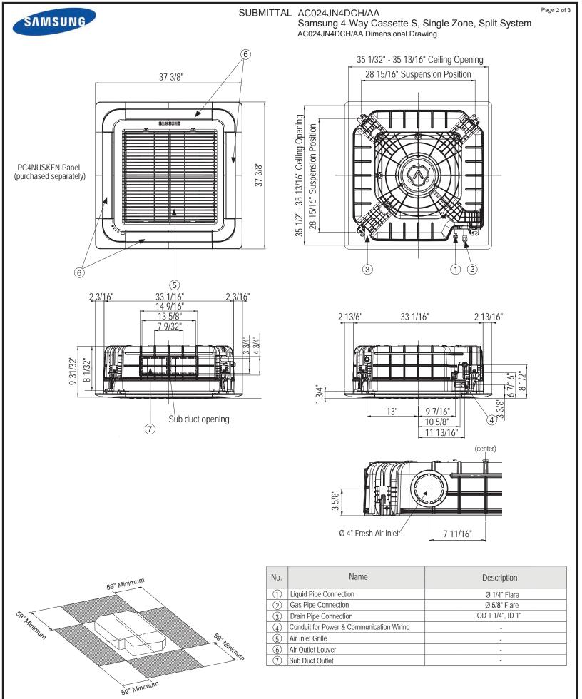
Proper clearance must be maintained around unit for proper operation.
