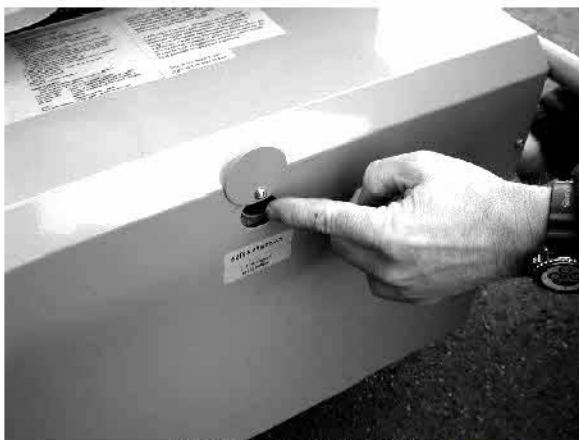
Press the Flame Control Reset Button
