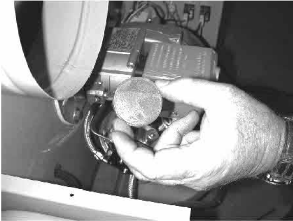
Remove the fuel pump screen
