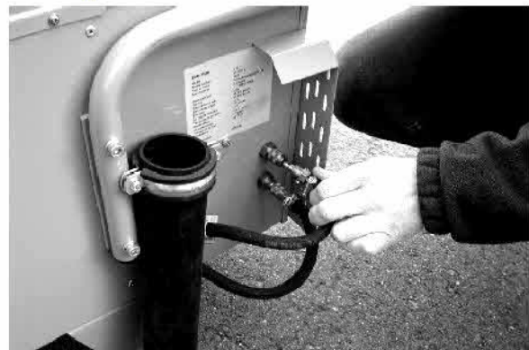
Connect the internal tank fuel lines
