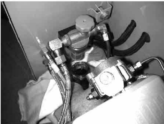
Unscrew the filter reservoir by hand
