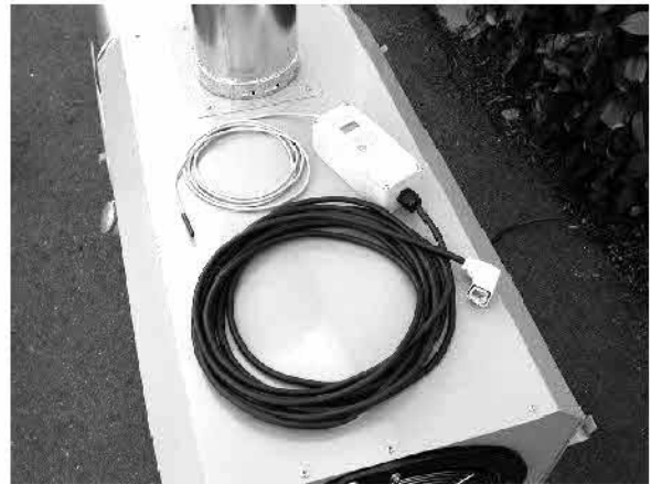
The remote thermostat sensor cable, control box, cable, and jack
