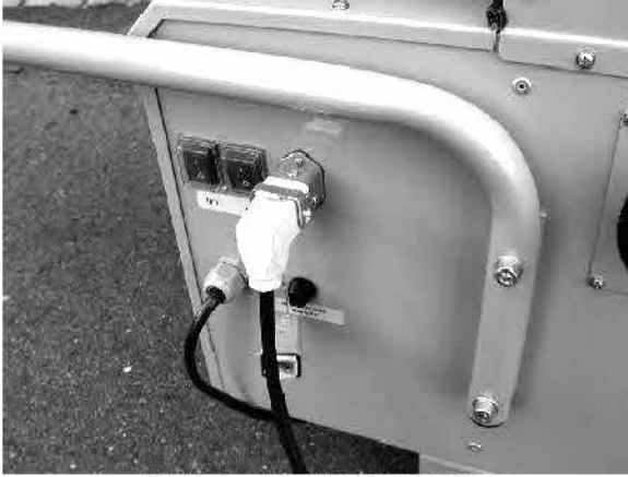
Plug the thermostat into the jack on the Dragon
