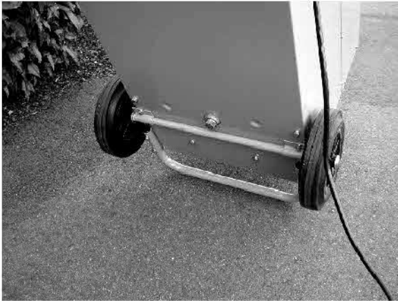
The internal fuel tank drain plug
