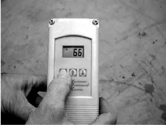
Before programming, the thermostat shows the current ambient temperature
