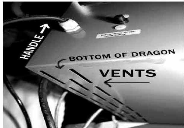
Air Intake vents shown from underneath unit.
