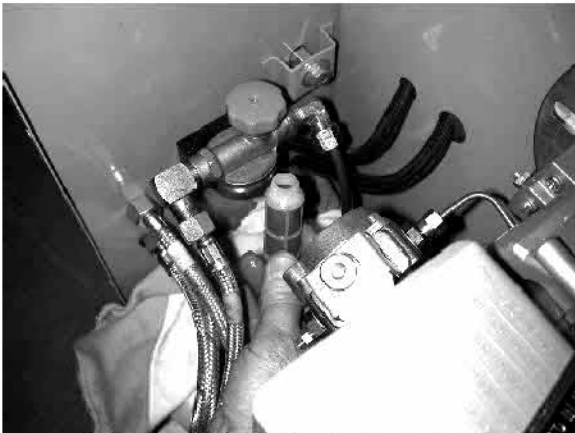
Unscrew the fuel intake filter by hand
