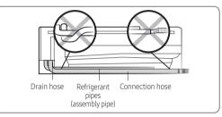
In Step 2-3, step 3 you determined the exit position for the piping bundle. The unit has three knockouts available for the left, right, and bottom exits. When the bundle exits directly from the rear, none of the knockouts are used.
