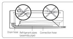
**3** Connect a 5/8-inch ID extension drain hose to the main drain hose.
