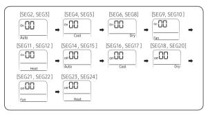
4 Save the option values into the indoor unit: Point the remote control to the remote control sensor on the indoor unit and then press the () (Power) button on the remote control twice. Make sure that this command is received by the indoor unit. When it is successfully received, you can hear a short sound from the indoor unit. If the command is not received, press the () (Power) button again.
