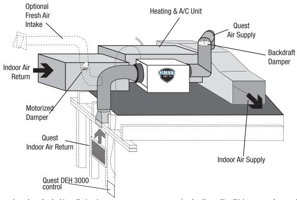
The preferred method of installation is to create a separate return for the Quest Dry 70 in a central area of the structure. Duct the supply of the Quest Dry 70 to the air supply of the existing HVAC system.
