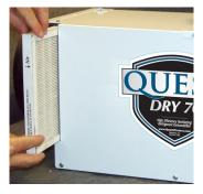
Replace filter door by inserting the bottom tab into the slot, aligning the door and pushing it gently against the unit until the snap button secures the door.
