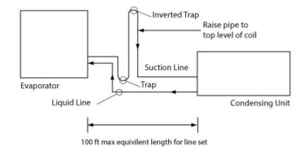
2. When the evaporator is located below the condensing unit, a suction trap must be installed at the evaporator, and an inverted trap must be installed at the condensing unit, for proper oil return, as follows:
