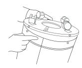
Using a #2 Philips screwdriver, install the four screws to hold the base onto the unit making sure the arrow on the sticker lines up with the unit's rear seam.
