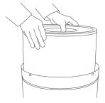
Place the HEPA & Activated Carbon filters inside on top of the gasket.
