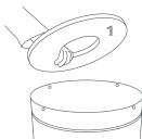
Place one gasket inside the unit all the way at the bottom.
