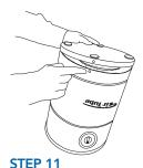
Place lid back to its proper position by aligning screw holes.
