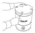
**STEP 12** With a screw driver, place 4 screws back into their positions.
