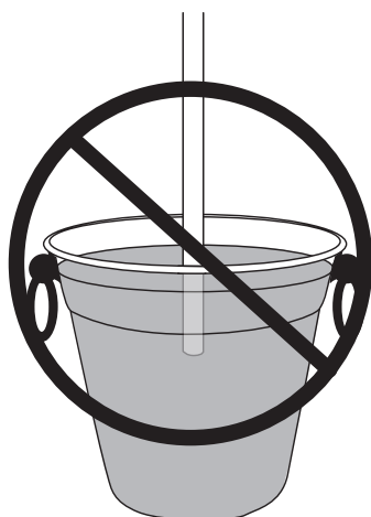
WRONG: Drain line is under water.
