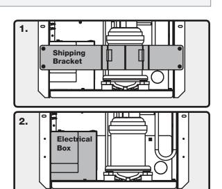
**Step 3.** There are three electrical knock outs, one on the back and two on the bottom of the unit. Remove appropriate knock out and install non-metallic cable clamp with clamp screws inside of unit oriented so they are accessible for tightening later.
