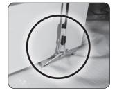
**Step 7:** Using the ratchet end of the ratchet strap, attach each strap to the eye bolts above the unit. If additional slack on the rope is needed, push the trigger on the ratchet end of the strap up and feed the rope through as needed.
