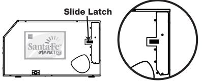
**Step 2:** Remove the filter by gently pulling it straight out of the unit. Insert new filter by gently pushing it straight into the unit. Make sure the AIR FLOW arrow on the filter is pointing into the unit.
