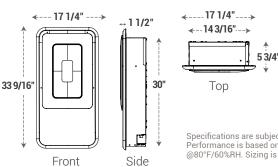
Specifications are subject to change without notice. Performance is based on pints / gallons per day @80°F/60%RH. Sizing is based on 10 foot ceiling height.
