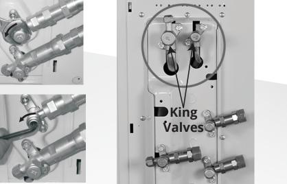
5. Using soapy water (in a spray bottle or with a brush), or leak detection spray, apply to the Quick Connect<sup>®</sup> fittings at the indoor air handler and outdoor condenser to check for leaks. If you see bubbles begin to form, this indicates there is a leak. If so, re-tighten the connection accordingly until the bubbles are gone. Please refer to the manual for more detailed information on checking for leaks.
