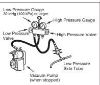
4) Leave the high pressure valve and the lowpressure valve of the gauge manifold closed for five min or more, and confirm that the gauge pointer does not return to zero.
