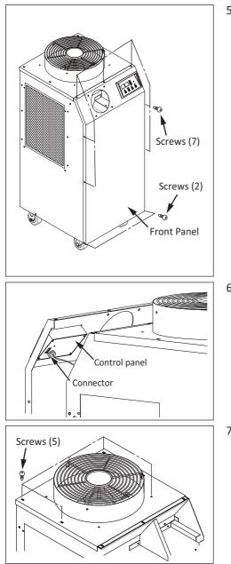
5) Take out the seven (7) screws. Unfasten two (2) screws to a half point. Pull the front panel forward.
