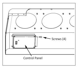
1) Take out the four (4) screws, and then remove the control panel.
