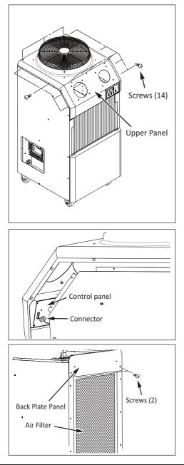
6) Take out the fourteen (14) screws, and then remove the upper panel.
