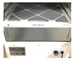
6. The weight of the cartridge and HEPA will keep everything in place, however the thumb screws along the inside rails can be tightened down slightly to prevent shifting in the event the unit is picked up and moved. Do not over tighten.
