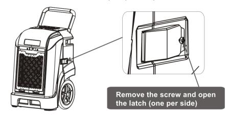
2. Undo the two latches on the base of the unit by pressing in the safety then opening the latch.
