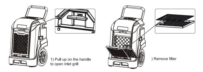
2. You can clean the filter by vacuuming it or rinsing it with warm water (no soap or solvents). Always make sure the filter is dry prior to restarting the unit.
