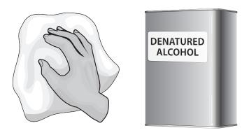
Should the reflective plates in the lamp chamber get dirty, carefully remove the UV lamps and stainless steel tube. Use a clean soft cloth and denatured alcohol to gently wipe them down; then, replace the lamps and tube.
