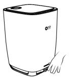
Gently pull the power cable out of the air inlet and connect the short extension cable with the local power plug.
