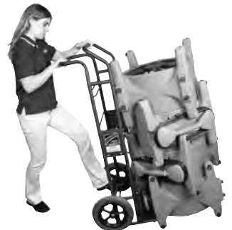
Ace Picture 4: Properly stacked Ace TurboDryers are now ready for transporting.
