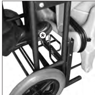
Ace Picture 2: Next, use foot to depress spring-loaded mechanism* on Unimover™.
