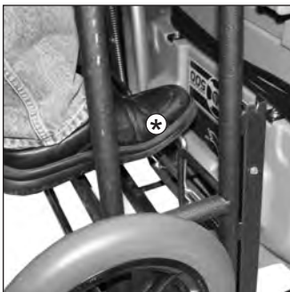
HEPA Picture 1: Stack up to 3 HEPA 500s. First depress spring-loaded mechanism* on Unimover.
