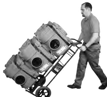
HEPA Picture 3: Properly stacked HEPA 500s are now ready for transporting.
