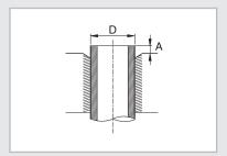
5 Check that the flaring is correct, referring to the illustrations below for examples of incorrect flaring.
