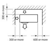
When 3 sides of the outdoor unit are blocked by the wall
