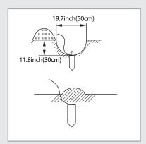
If the power distribution circuit does not have a grounding or the grounding does not comply with specifications, an grounding electrode must be installed. The corresponding accessories are not supplied with the air conditioner.
