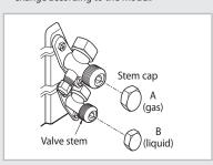
The air in the indoor unit and in the pipe must be purged. If air remains in the refrigeration pipes, it will affect the compressor either reduce cooling/heating capacity or lead to a malfuction. Refrigerant for air purging is not charged in the outdoor unit. Use Vacuum Pump as shown at the right figure.
