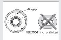
Once you have checked that there are no leaks in the system, you can insulate the piping and hose.
