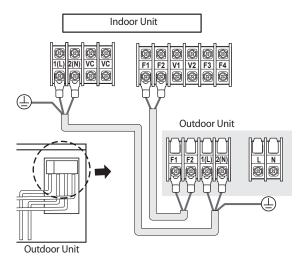
Ground wire for the indoor unit and outdoor unit connection cable must be clamped to a soft copper tin-plated eyelet terminal with M4 screw hole(NOT SUPPLIED WITH UNIT ACCESSORIES).
