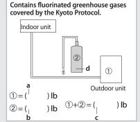
The filled-out label must be adhered in the proximity of the product charging port (e.g. onto the inside of the stop valve cover).
