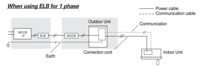
\* If an outdoor unit is installed in a place in danger of an electric leak or submergence, you must install the ELB.
