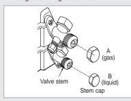
The air in the indoor unit and in the pipe must be purged. If air remains in the refrigeration pipes, it will affect the compressor, reduce to cooling capacity and could lead to a malfunction. Refrigerant for air purging is not charged in the outdoor unit. Use Vacuum Pump as shown at the figure.
