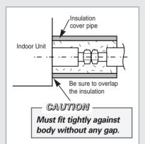
3 Finish wrapping insulating tape around the rest of the pipes leading to the outdoor unit.
