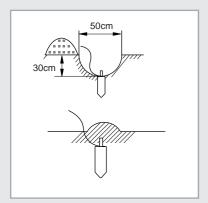
If the power distribution circuit does not have an earth or the ground does not comply with specifications, an grounding electrode must be installed. The corresponding accessories are not supplied with the air conditioner.
