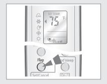
You can adjust the airflow direction vertically. The outer airflow blade moves up and down to increase the efficiency of the cooling or heating operation.
