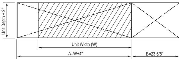
In applications where there is not a tile ceiling, an inspection hole is required.
